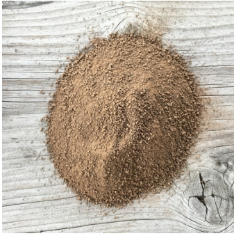
(c) Silt Loam. Expected c = 60 - 90kPa and 25^\circ \leq \phi \leq 32^\circ .
