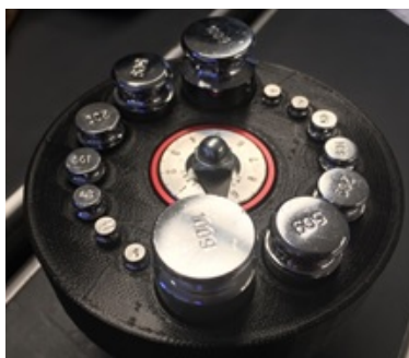
Fig. 3: Modified pocket shear vane tester including: a 3D printed cast with weight slots; calibration weights.
