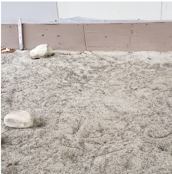
(a) Sand pit in which tests were performed. Expected values are c = 0kPa and \phi = 37^\circ - 38^\circ .
