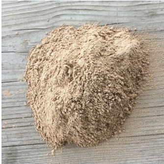
(a) Dry clay of low plasticity. Expected c = 86kPa and 27^\circ \leq \phi \leq 35^\circ ,
